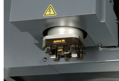
Supports parallel electrode setup and index machining Supports fluid emission from spindle center (photo shows 3R-MACRO chuck specifications)
