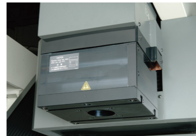
Prepare two T-slots and electrode mounting table installation screw (photo shows EA28V ADVANCE specifications)
