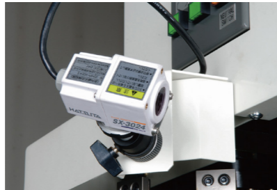
Catches infrared rays from flames and stops power supply
